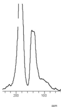
Single pulse 17 O MAS NMR of Ba 2 In 2 O 5 @ 122 MHz (900 MHz rel. 1 H) with a spinning speed of 22 kHz
