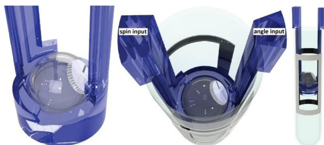
Figure 1: Computer-assisted design of 6 mm spherical rotor in the MAS-insert, with the spin and angle-adjust pneumatic inputs called out (center), and the unit inserted in 10 mm solution-state tube (right).
